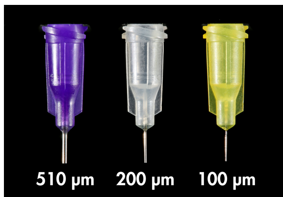
Figure 3.10: The three syringe tips used in the microextrusion experiment. The labels refer to the inner diameter of the steel tubes.
